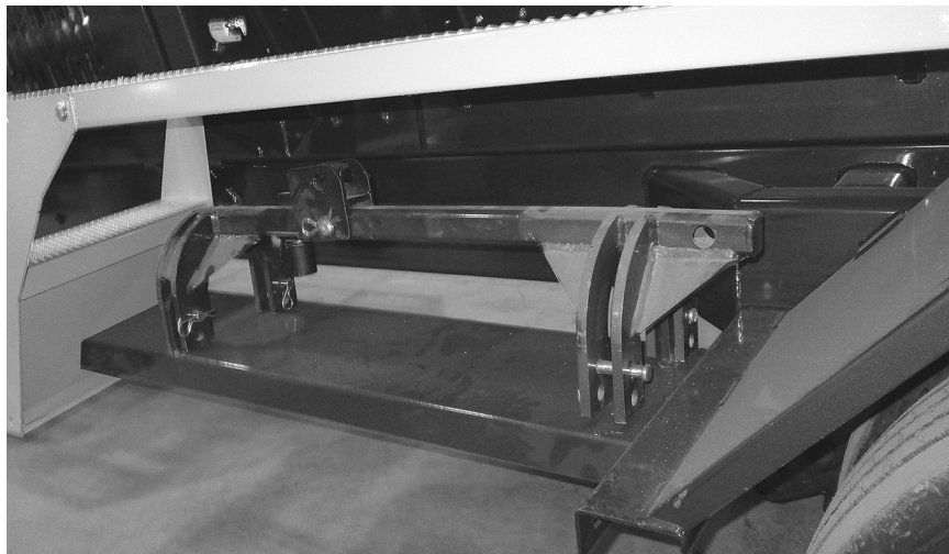
Hydraulic hammer rod puller storage
