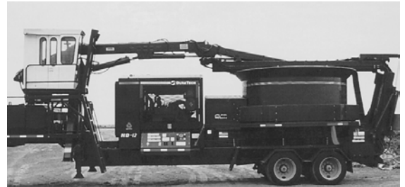
cab and grapple loader shown in the transport position on the HD-12
