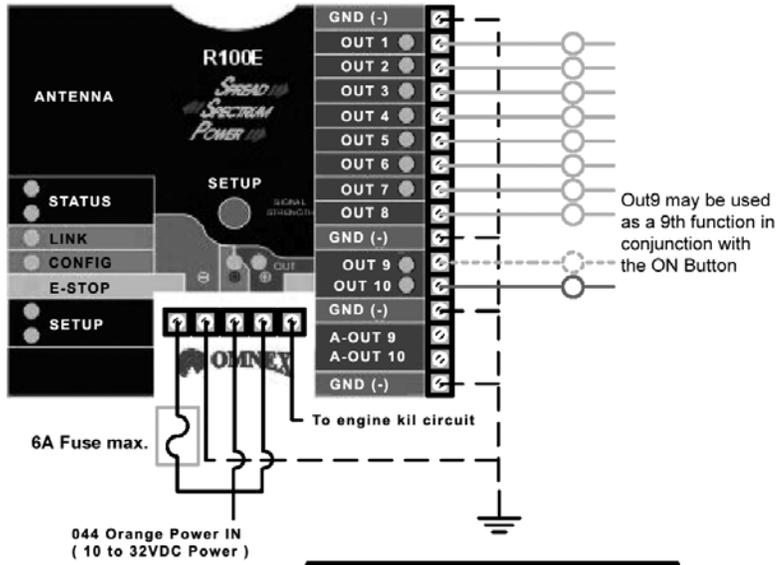
**NOTE:** Although the Outputs are rated at 10A, the [E-Stop] relay is only 6A and therefore must be fused appropriately
