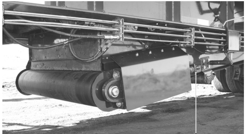
belly conveyor tail pulley tensioning bolts
