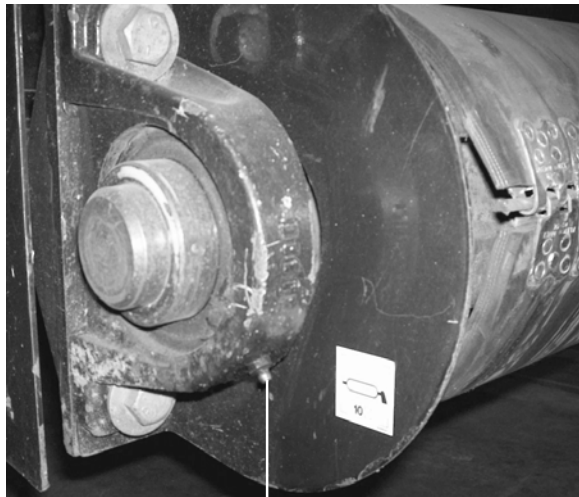
belly conveyor tail pulley bearing (ref # 12)
