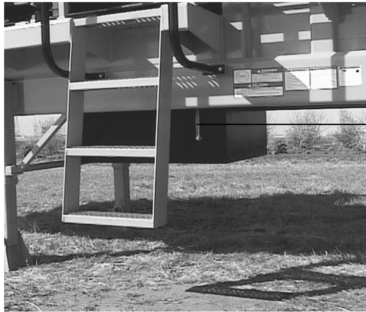
fuel level sight glass
