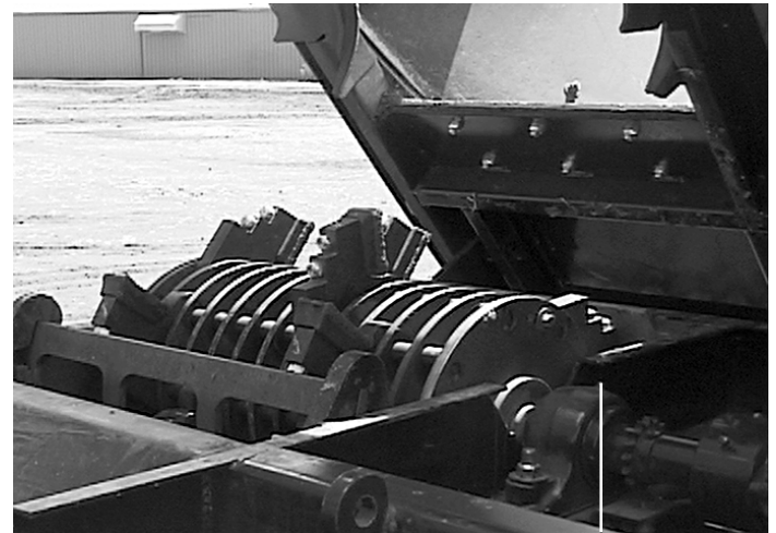
rotor bearing lubrication zerk (ref 3)
