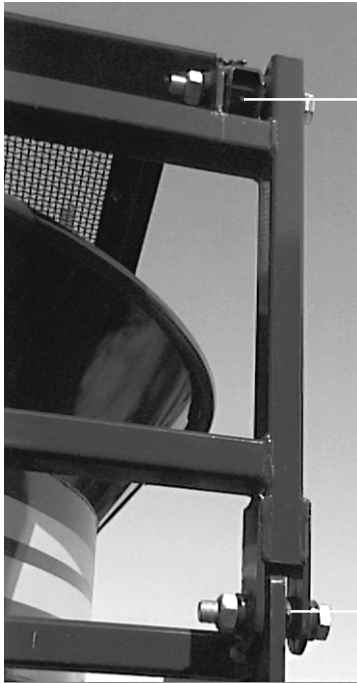
figure 5.3 optional tub cover lubrication points (left), tub tilt pivot point lubrication (right)
