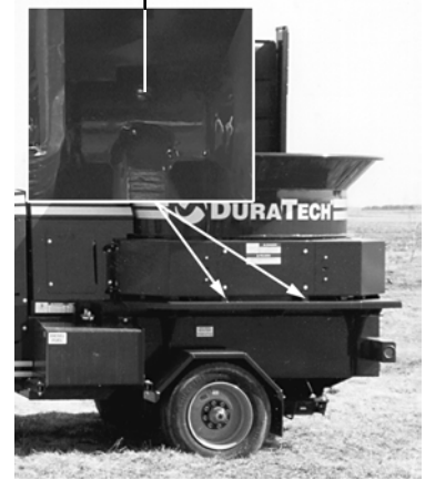
tub pivot, 50 deg. tub tilt - lubrication zerks (ref 6)
