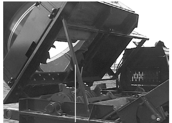
platform safety stop
