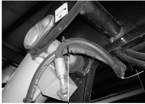
upper discharge conveyor lift cylinder (ref # 11)
