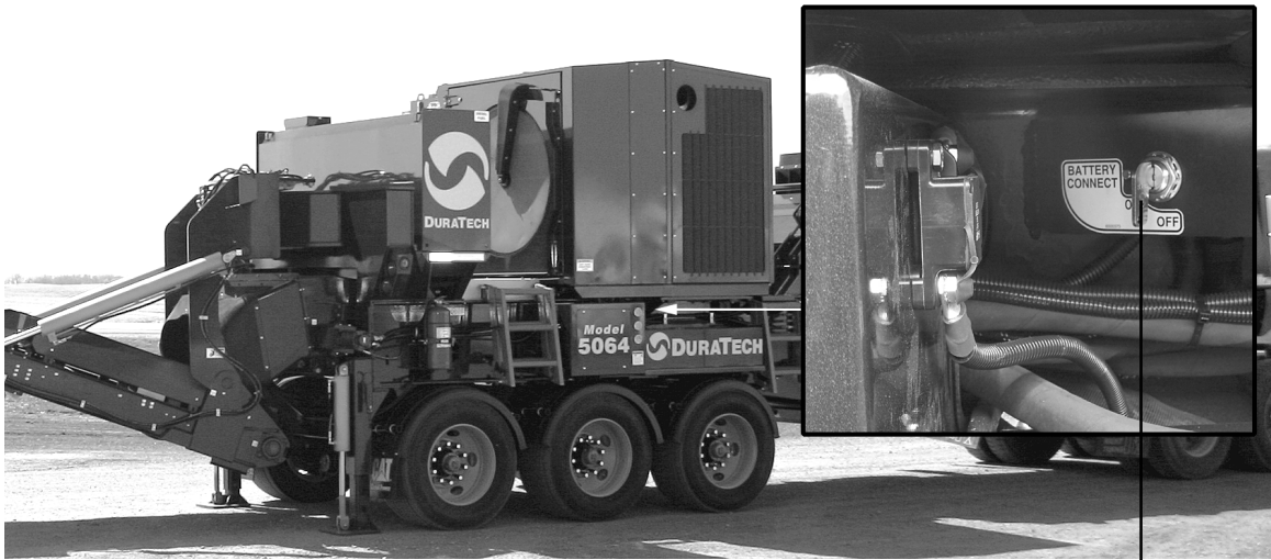
battery disconnect switch
