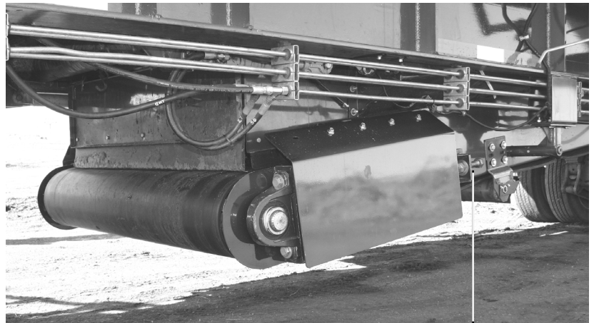
belly conveyor tail pulley tensioning bolts
