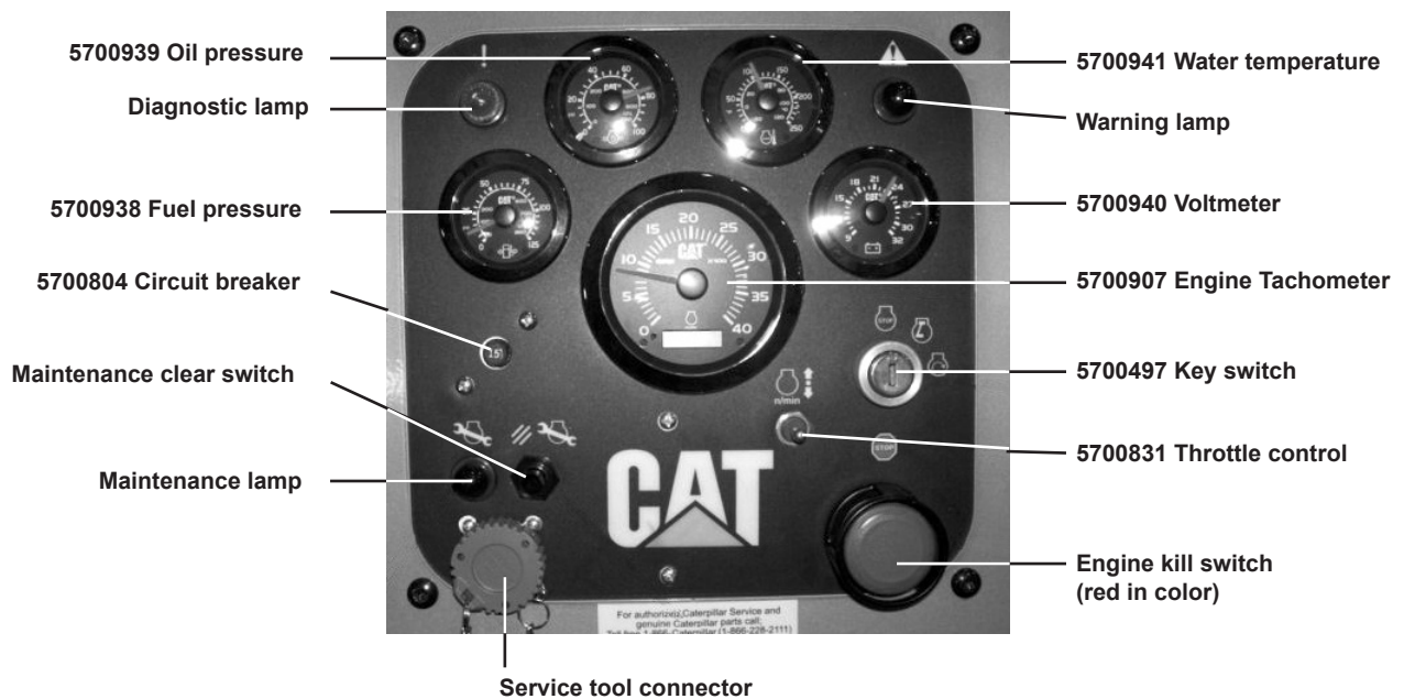
figure 2.7 Cat control panel for tier III engines
