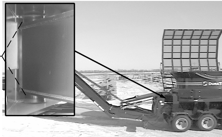
discharge conveyor swing pivot (Ref # 10)
